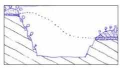
Scenario 2 (B) illustrates how 'top down' extraction allows the exposed vertical surface ('the working face') to be partially covered with soil placed on a 'bench'. This forms a growing medium for trees and shrubs that can begin to establish and mature while the next, lower, layer of the quarry is being developed.
