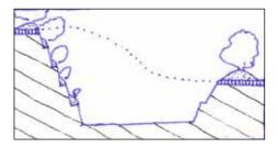
Fig 10.1 also illustrates how the adoption of gradual and on-going restoration coupled with "top down" extraction allows extraction to continue with minimal visibility of either the working faces or the equipment. The resultant profile of the quarry illustrates how it will be much more easily assimilated into the form of the existing landscape, especially once planting becomes mature.
